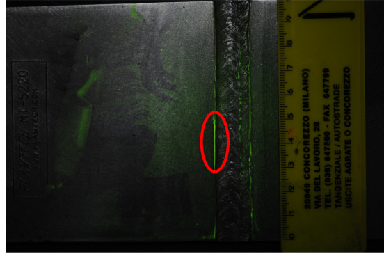
Picture 1B Specimen number MT-5220 Flawtech Fluorescent Magnetic Powder Elite FW1 UV Light: 3.000\mu\text{W}/\text{cm}^2 Visible Light: 500\text{ lx}
