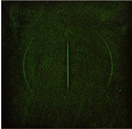
Picture D 1 Fluorescent Magnetic Powder Elite FW1 UV Light: 1.500\mu\text{W}/\text{cm}^2 Visible Light: < 20\text{ lx}
