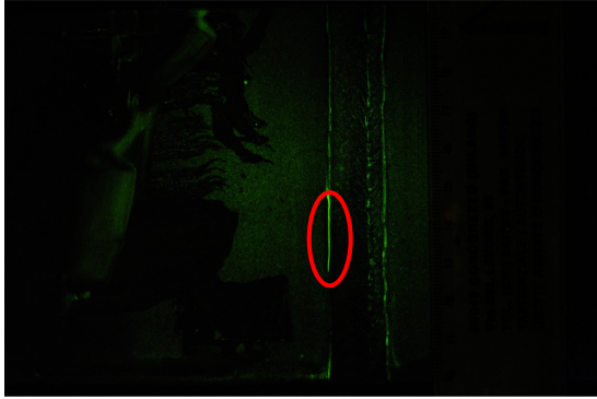
Picture 1A Specimen number MT-5220 Flawtech Fluorescent Magnetic Powder Elite FW1 UV Light: 1.500\mu\text{W}/\text{cm}^2 Visible Light: < 20\text{ lx}
